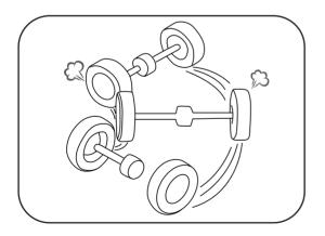
**NOTE**: Oil in differential should be checked and replaced in 180-day maintenance period. Permanent damage might arise if it is not replaced.
